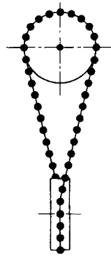
Fig. 3—Skewed shafts normally acquire two sets of spiral gears to bridge space between shafts. Angle misalignment does not interfere with qualified bead chain operation on sprockets.
